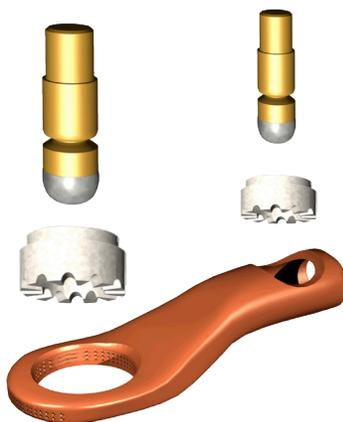
This cable lug is both PinBrazed to the cable and to the surface. No crimping tool is needed. The cable is inserted in the lug which is flatten and the cable is then PinBrazed to the lug by placing the brazing pin in the flattened hole.
